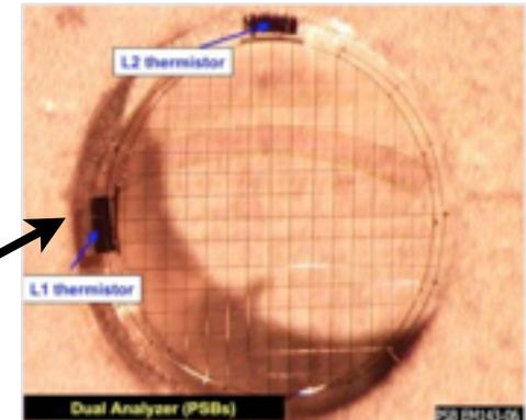
Derivation of Stokes parameters (I, Q and U) involves the combination of two pairs of PSB bolometers that observe the same sky positions within a few seconds. The polarizers of the second pair are rotated by  $45^\circ$  with respect to the first pair.
